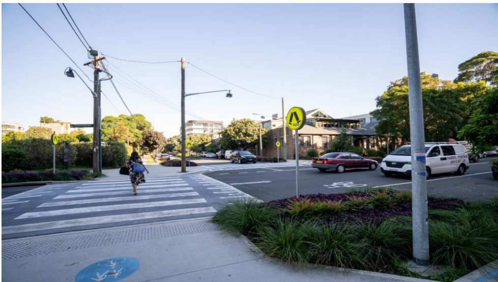
Figure 4.3 Rothschild Ave, Rosebery at the intersection with Cressy Street- Wombat crossing example.
